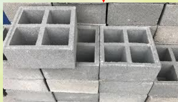
VENTILATION BLOCK (STAIRCASE WALL)
